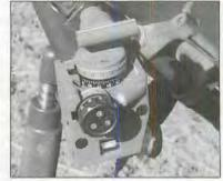
The lensatic version of the South African H-019 mortar sight includes a number of important features. There is a quick-release dovetail interface for rapid installation and removal from the weapon. There are double bubbles for leveling in each plane. All the scales and bubbles are equipped with selfluminous tritium illumination that can be covered when not in use. The optical sighting device can be adjusted in the vertical plane and is also provided with a betalight.
